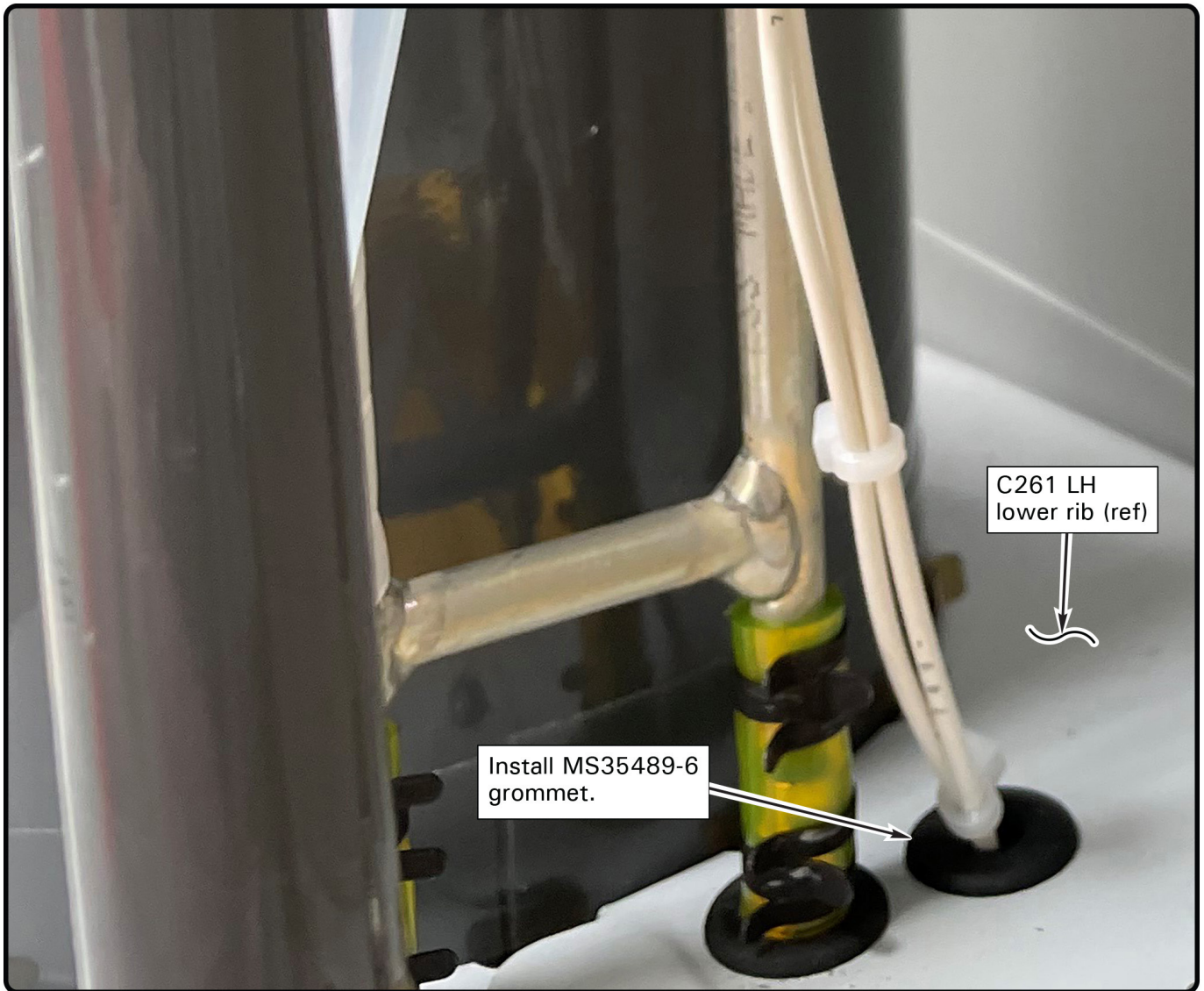
Image 2 Grommet installation (view looking aft from helicopter RH side)
