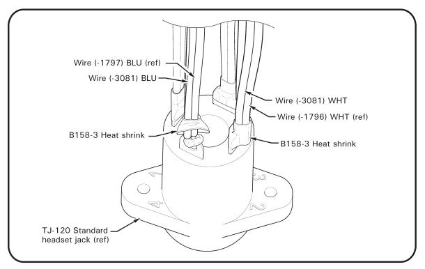
FIGURE 1A Solder splice at TJ-120 jack
