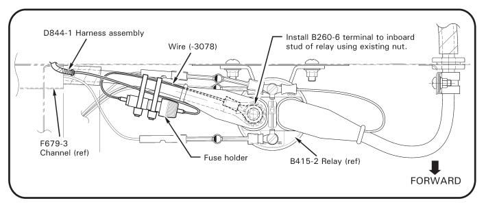
FIGURE 4A Installing & securing fuse holder (Battery relay; view looking down)
