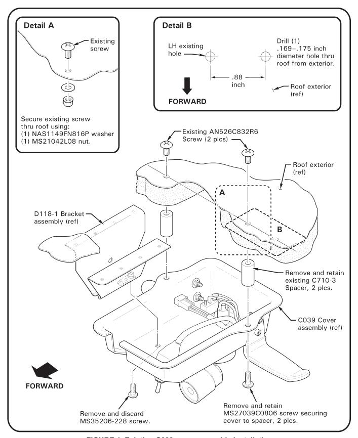
FIGURE 1 Existing C039 cover assembly installation
