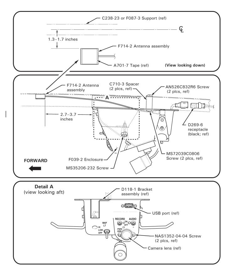
FIGURE 2 Camera enclosure and antenna installation
