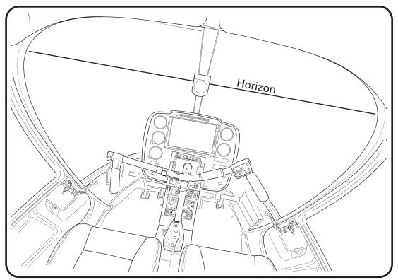
FIGURE 3 Camera view angle (angle shown requires adjustment)
