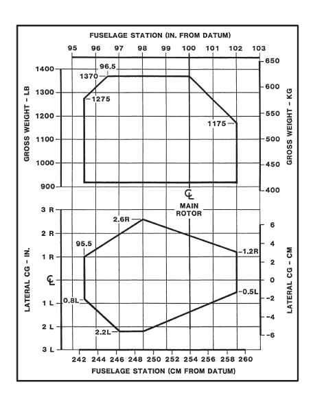
R22 ALPHA, BETA, AND BETA II CENTER OF GRAVITY LIMITS
