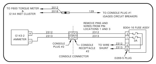
FIGURE 2A Existing schematic
