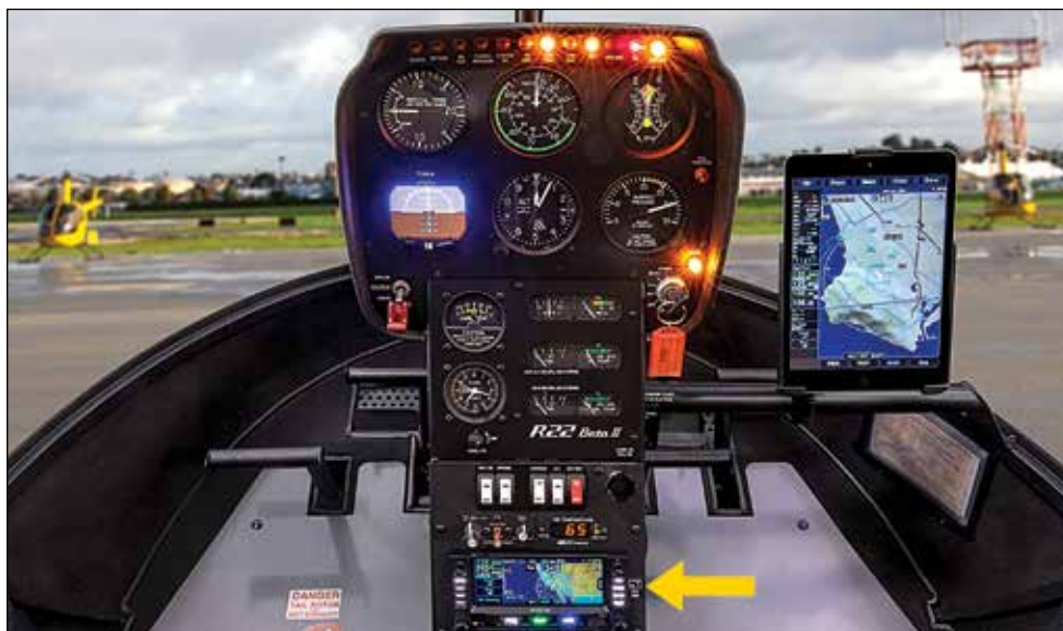
Avidyne IFD 440 installed in center console and wirelessly connected to iPad on accessory bar.
