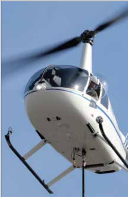
*The cargo hook installation allows for solo flight from either seat.*
