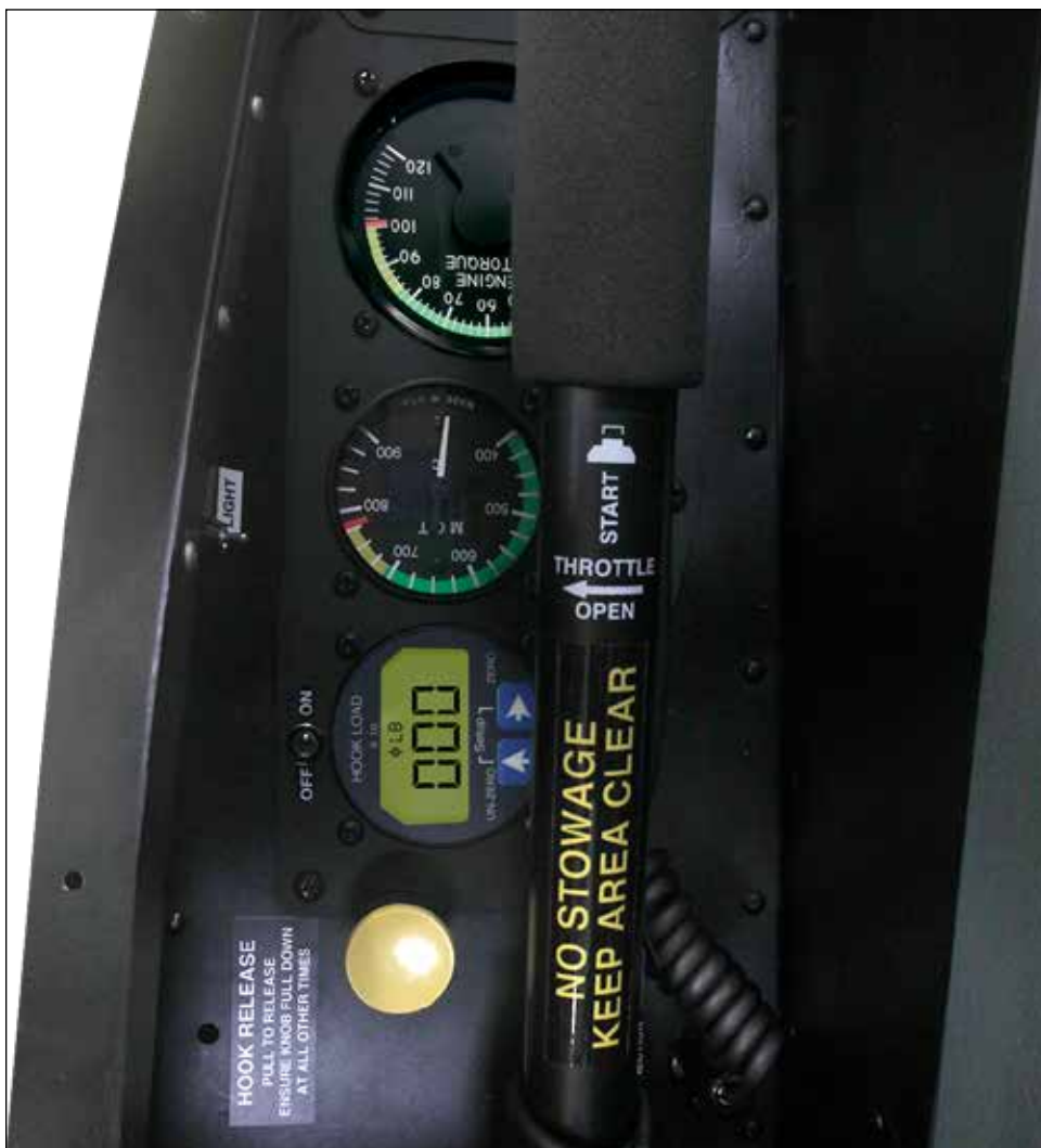
Left door sill panel contains supplemental engine torque and gas temperature gages, a load cell display, and an emergency manual hook release.
