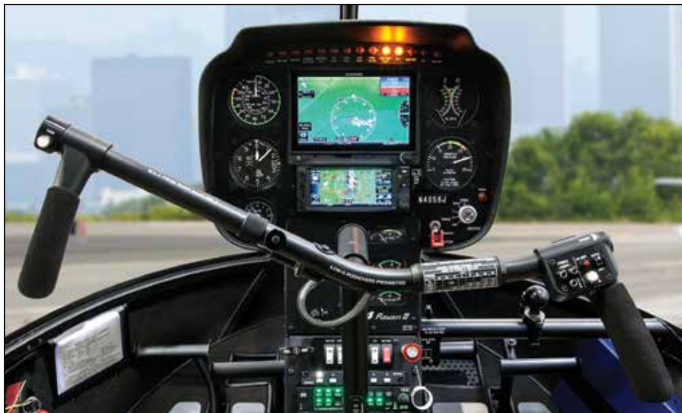
R44 with Garmin GDU 700L TXi display installed in the new compact instrument console.
