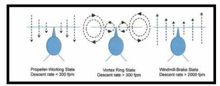
In the propeller working state, air moves down through the rotor. At a descent rate greater than 300 fpm, the vortex ring state begins; some downflow moves radially out under the rotor disc and is drawn up and into the rotor. In the windmill brake state, all air moves up through the rotor.
