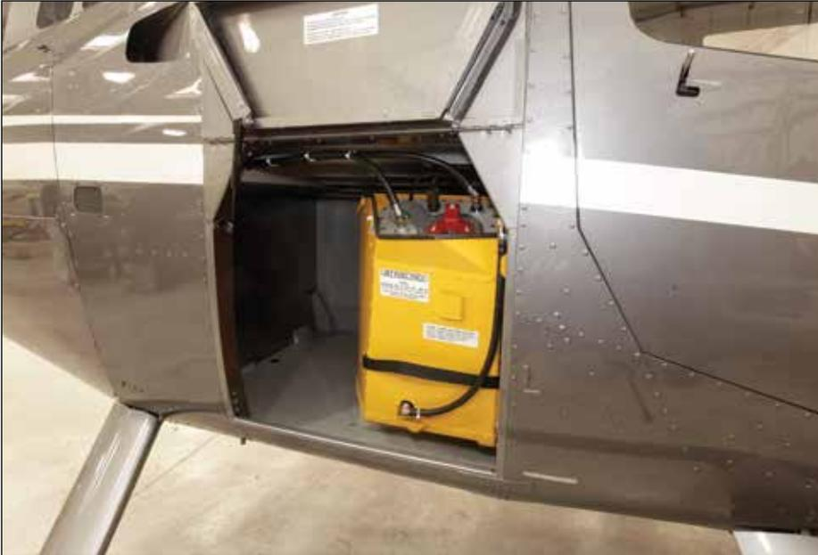
Auxiliary fuel tank installed in R66 baggage compartment.
