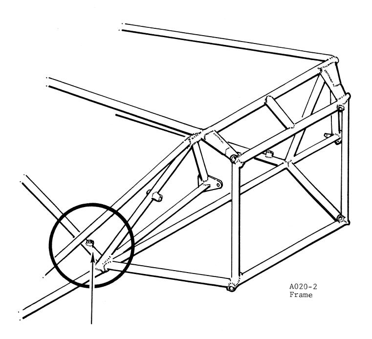
Inspect for Cracks
