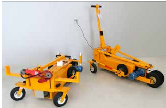
MT950 tow cart with optional kits attached (left) and standard MT950 (right)
