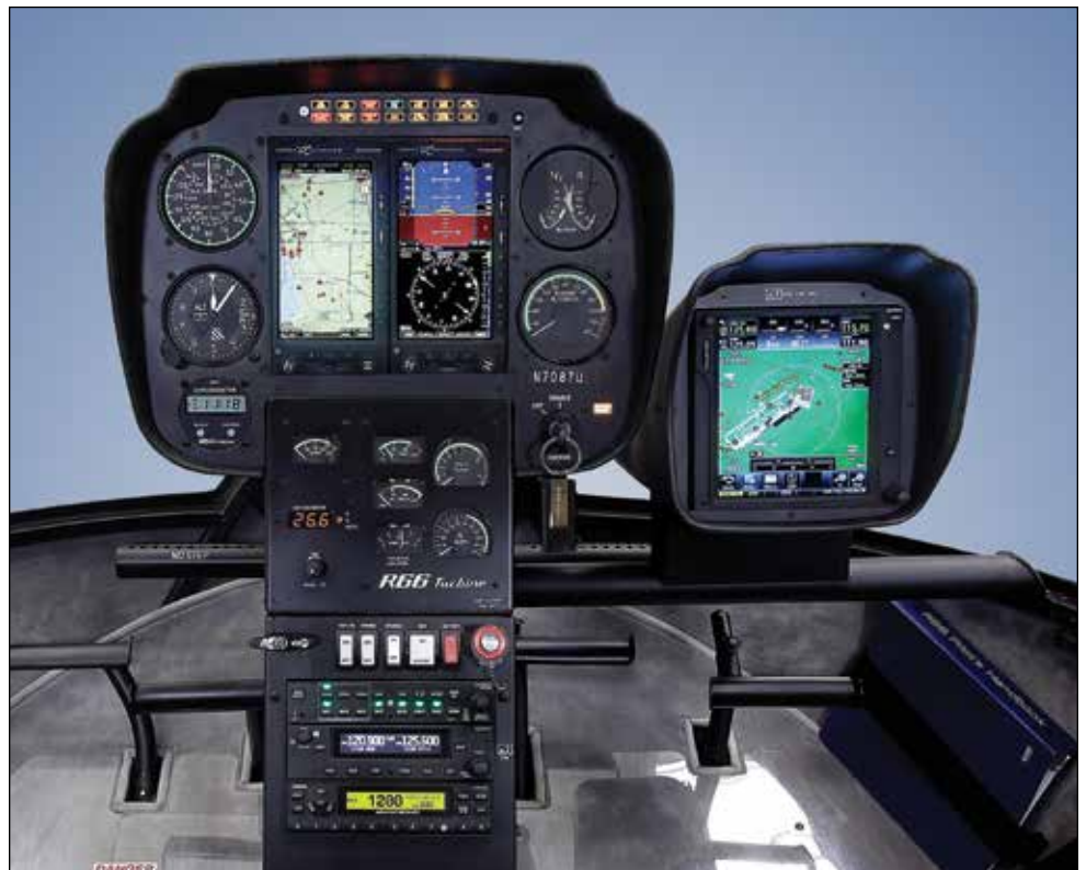
Eight-hole instrument panel with Aspen Avionics EFD500H MFD (left) and EFD1000H PFD (right). Pilot side console (PSC) holds Garmin GTN 750 GPS/COM/NAV.
