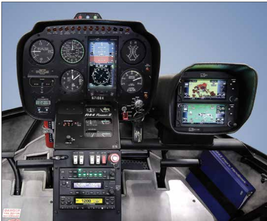
Eight-hole instrument panel configured with Aspen EFD1000H PFD. Pilot side console houses Garmin GTN 625 GPS (top) and GTN 635 GPS/COM (bottom).
