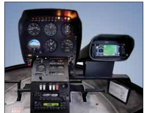
Six-hole instrument panel in R22 with Garmin 625 GPS in PSC.
