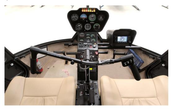
Original 7-Instrument Console with Pilot Avionics Console
