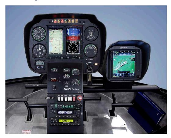
8-Instrument Console with Pilot Avionics Console
