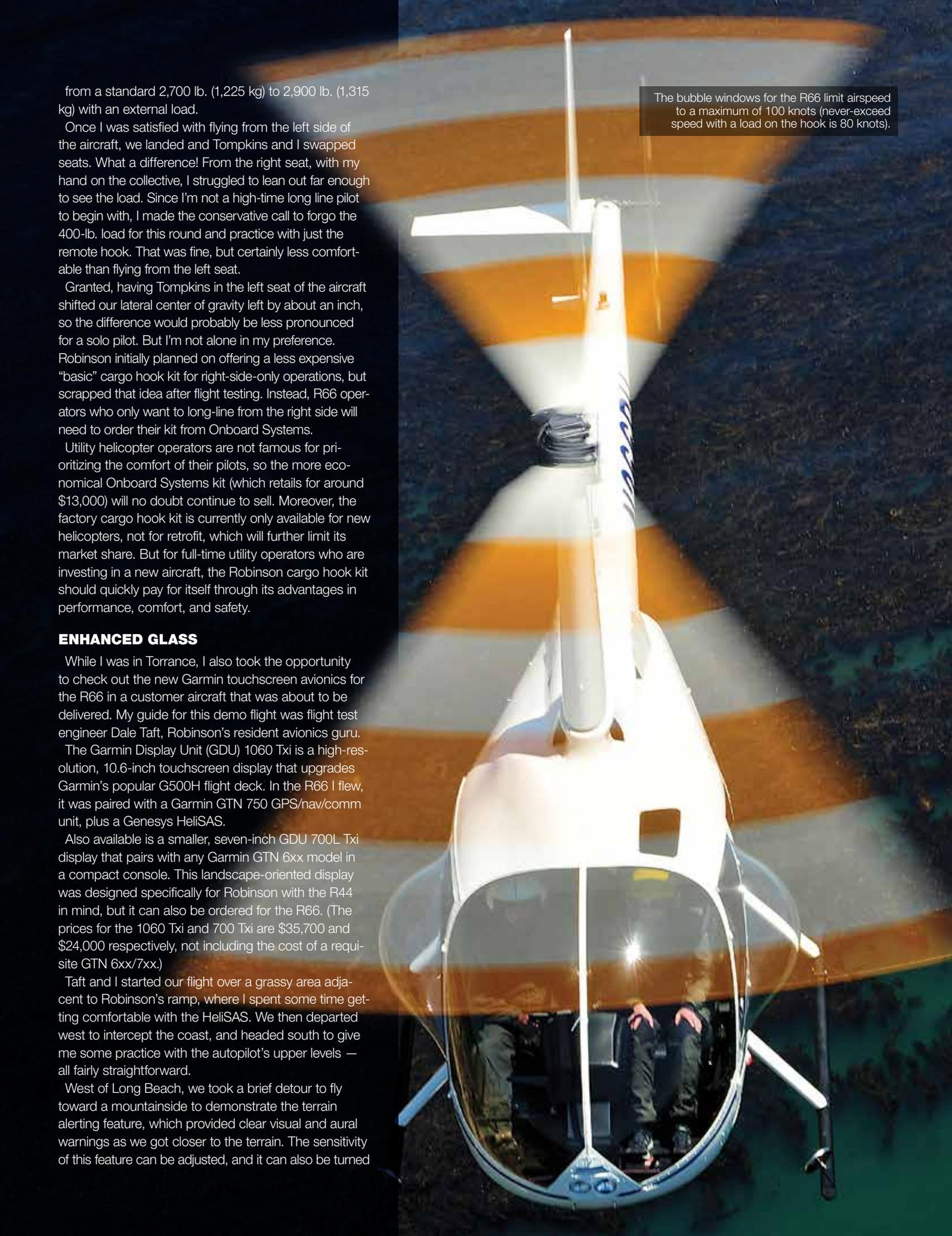
The bubble windows for the R66 limit airspeed to a maximum of 100 knots (never-exceed speed with a load on the hook is 80 knots).
