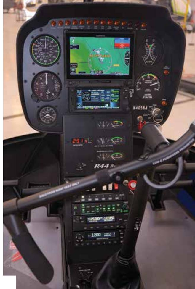
1 // At left, an R66 panel featuring the 10.6-inch Garmin Display Unit 1060 Txi. A smaller seven-inch GDU 700L Txi is also available, shown here at right, installed in an R44. 2 // While the 1060 Txi panel takes up more space than it strictly needs to, pilots who learned on steam gauges will likely feel comfortable with the analog redundancy.
