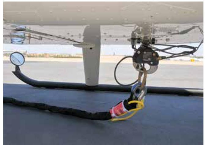
once. The bubble windows limit never-exceed speed (Vne) to 100 knots indicated airspeed (Vne with a load on the hook is 80 knots). When we later did a photo shoot with both bubble doors but no line on the hook, the aircraft reached 100 knots easily, with no adverse vibrations.
