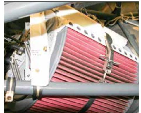
Inlet Barrier Filter installed in R66
