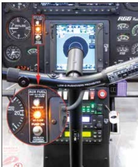
Controls are located on the R66 instrument panel
